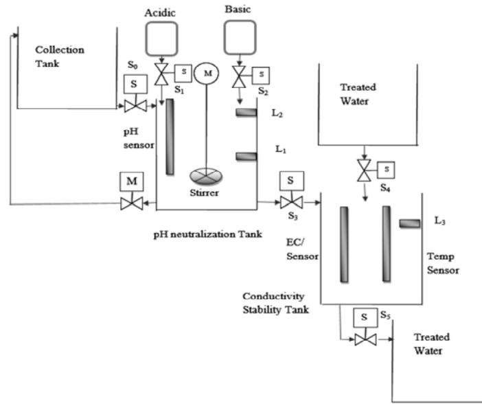
**Fig. 3: Schematic diagram of the proposed system**
