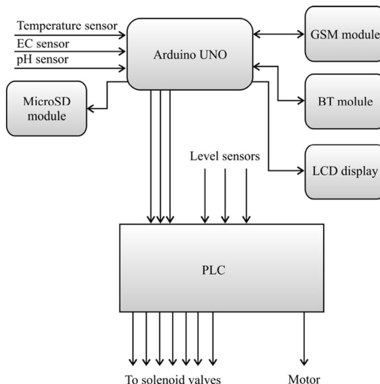
**Fig. 1: Block diagram of the automated system**
