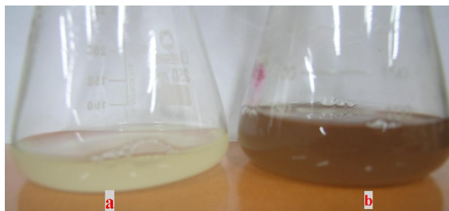
Figure 1 : Fungal filtrate with silver ion (a): Control flask, (b): After 24 hrs of reaction
