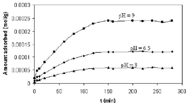
**Figure 3 :** Effect of solution pH on NMB adsorption on mordenite nanocrystal zeolite. Adsorption conditions: 0.05 g adsorbent, NMB initial concentration:  $1.00 \times 10^{-5}$  M, temperature: 25 °C.
