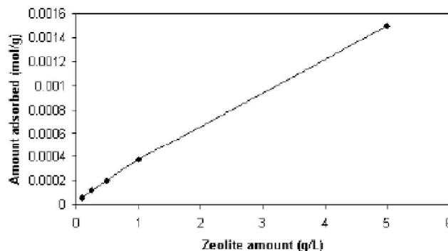
**Figure 5 :** Influence of mordenite nanocrystal zeolite amount on the adsorption amount of NMB.
