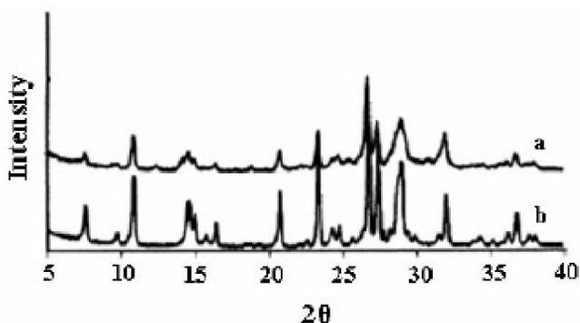
Figure 1 : XRD patterns of (a) mordenite nanocrystal zeolite (b) mordenite zeolite.
