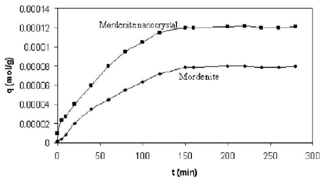
Figure 2. Comparison of dynamic adsorption of NMB on mordenite nanocrystal and mordenite zeolite. Adsorption conditions: 0.05 g adsorbent in 200 mL NMB initial concentration  $1.00 \times 10^{-5} \text{ M}$ , temperature:  $25^\circ \text{C}$ , pH = 6.5.
