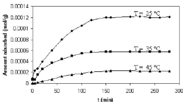
**Figure 4 :** Effect of solution temperature on NMB adsorption on mordenite nanocrystal zeolite. Adsorption conditions: NMB initial concentration:  $1.00 \times 10^{-3}$  M, pH = 6.5.
