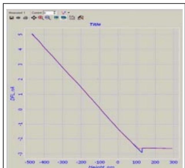
Figure 8: force curve obtain by CSG01 cantilever in contact mode
