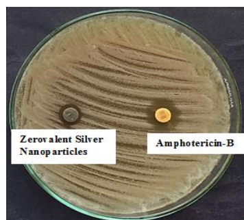
FIG. 5. Zone of inhibition test for antibacterial activity of silver nanoparticles against P. aeruginosa .
