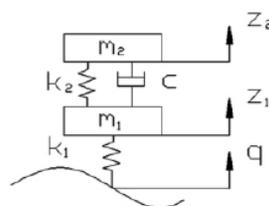
Figure 3 : Vehicle unilateral front wheel vibration system
