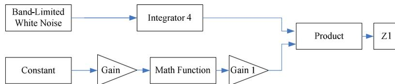
**Figure 4 : Finite bandwidth white noise road excitation model**
