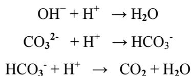
Alkalinity is significant in the treatment of waste water and drinking water, because it will influence treatment processes such as anaerobic digestion. Alkalinity is reported in units of mg/L  $\text{CaCO}_3$ , because the carbonate ion ( $\text{CO}_3^{2-}$ ) is its primary constituent. Total alkalinity is the sum of the phenolphthalein alkalinity and the methyl orange alkalinity. The desirable limit of total alkalinity is 200 mg/L (ICMR). The value of study area ranged from 90 to 310 mg/L.
