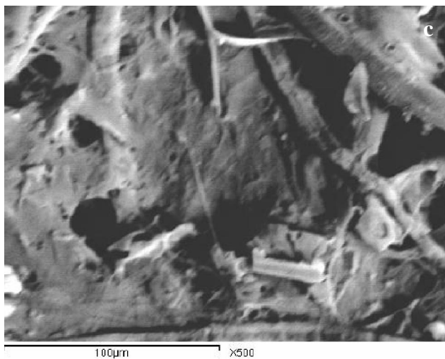
Figure 3 : Scanning electron micrographs of the surface of hand sheets of 50% rice straw pulp + 50% ONP type1 (a), 50% rice straw pulp + 50% ONP pulp type2 (b) and ONP type2 (c)
