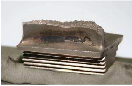
Figure 1 : Broken turbo blade
