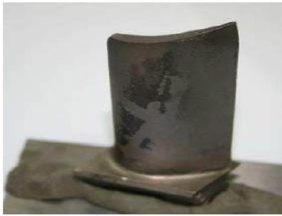
Figure 3 : Partially broken blade at the tip of the airfoil
