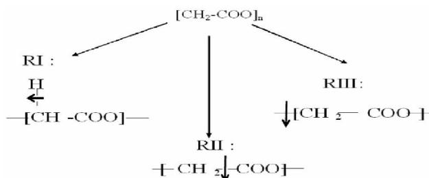
Figure 1 : Molecular structure of PGA and the most probable free radicals formed.
