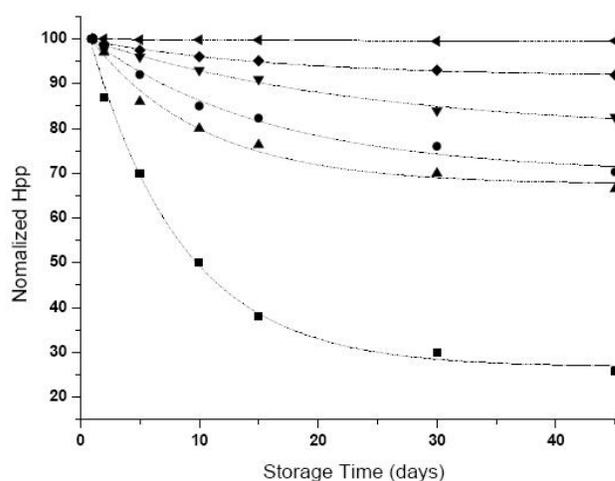
Figure 5 : Variations of the ESR signal intensity with storage time for PGA samples irradiated at a dose of 25kGy and kept at different temperatures: RT (■), 333K (▲), 353K (●), 373K (▼), 393K (◄), 413K (◆); calculated by a function describing first-order kinetic (dashed lines).
