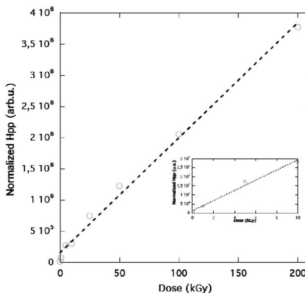
Figure 3 : Dose response curve of PGA dosimeter in the dose range of 0.1–200 kGy, experimental (°) and calculated by a linear function (dashed line).
