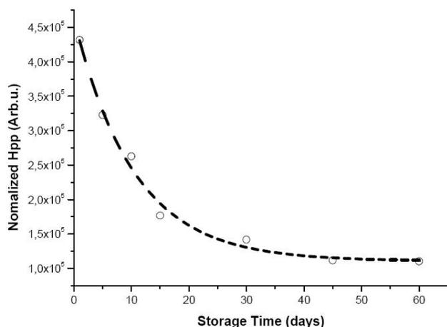
Figure 4 : Experimental and calculated ESR signal intensity decay curves for PGA irradiated at a dose of 25kGy and kept at room temperature. Symbol (experimental) and dashed line (theoretical, calculated by a function describing first- order kinetic).
