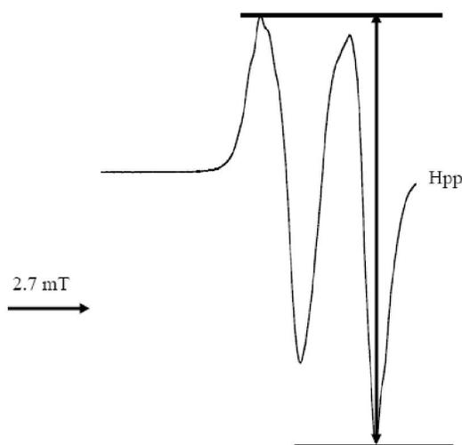
Figure 2 : Peak to peak higher (Hpp) of ESR spectra related to PGA irradiated at a dose of 25 kGy.
