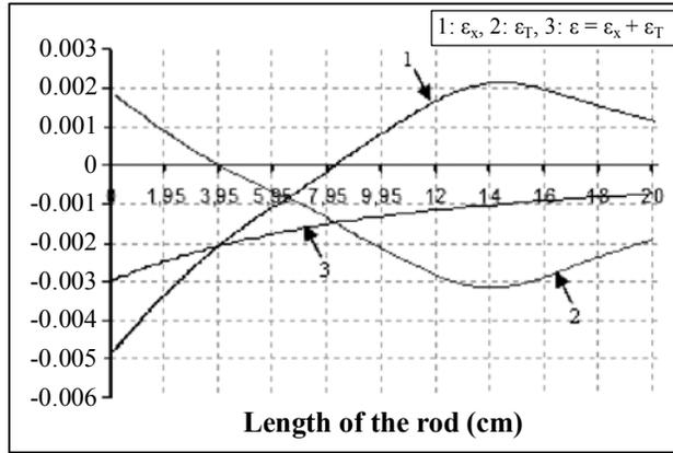
Fig. 2: Field distribution component deformations at  $T(x = 0) = T_1 = -150$  (°C)
