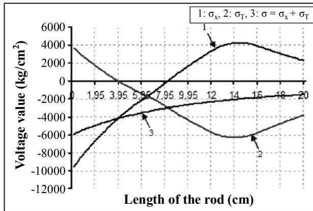
Fig. 3: Field distribution of stress components at  $T(x = 0) = T_1 = -150$  (°C)
