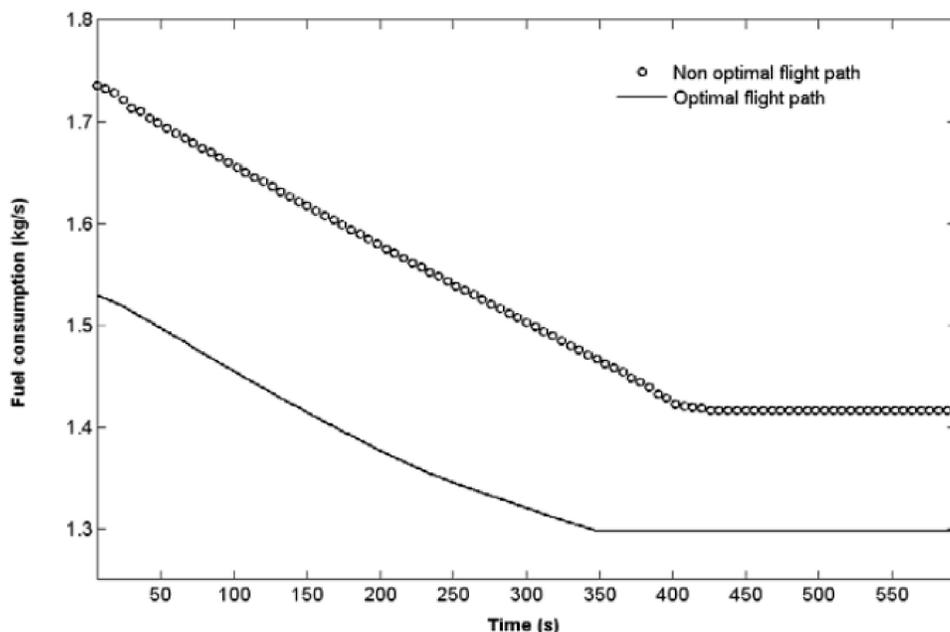
Figure 4 : Fuel consumption during approach
