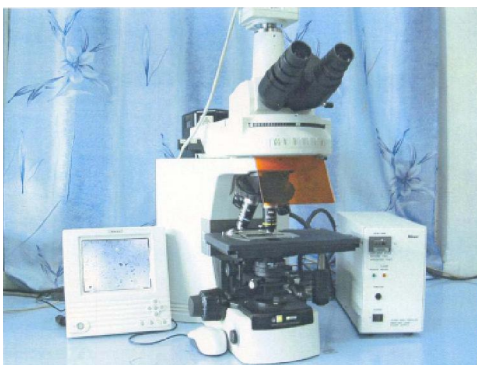
Figure 2 : A view of tri-nomial microscope (Make: Nikon, Japan) used for examination and identification of house desk mites
