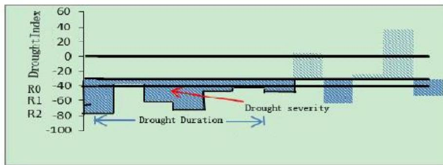
Figure 2: The identification of drought and the determination of drought variables
