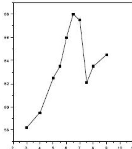
**Figure 6 : Effect of initial pH on the adsorption of chromium ion. [Cr]=30mg/L; Adsorbent dose=50mg/50ml; contact time=60min**
