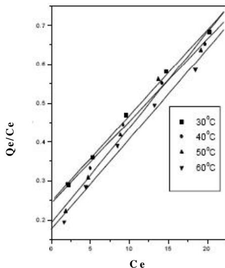
Figure 3 : Langmuir adsorption isotherm for the removal of chromium ion
