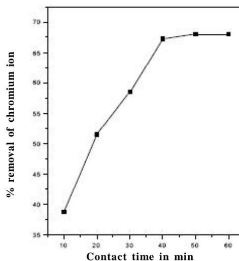
Figure 1: Effect of contact time on the adsorption of chromium ion. [Cr]=30mg/L; Adsorbent dose=50mg/50ml; pH=7
