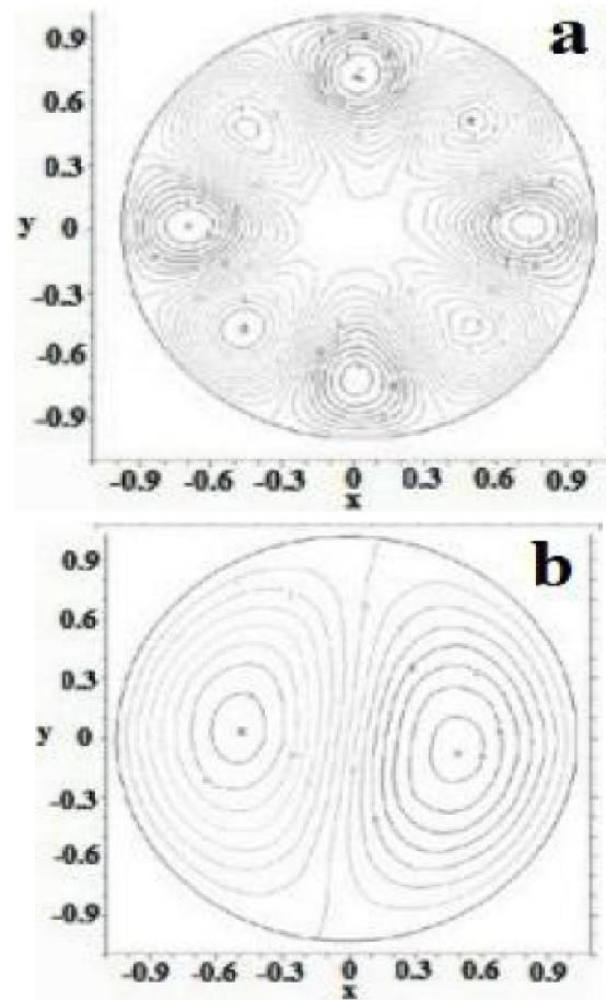
**Figure 4 : Frames of video filming from Figure 3c and Figure 3b, and calculated normal modes of vibrations of air in the cylinder, a – the 36<sup>th</sup> mode, b– the 4<sup>th</sup> mode**
