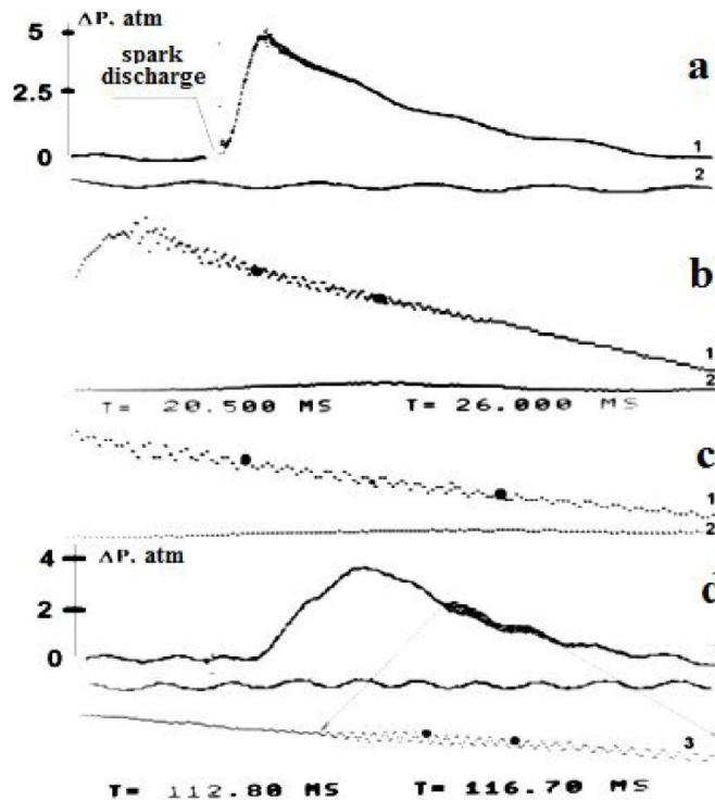
**Figure 2 :** Oscillograms of pressure change in combustion ignition of gas mixtures; 1 – signal at the initiated ignition; 2 – comparison signal, large black points – time interval; 3 – the stretched time interval; a,b,c – (H<sub>2</sub>+air)<sub>stoich</sub>, various time intervals; d – 15% H<sub>2</sub>+air + 3% CCl<sub>4</sub>
