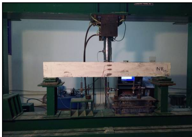
Fig. 2: Test setup of the control beam
