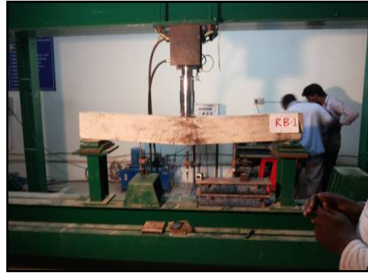
Fig. 5: Cracking pattern of RB specimen
