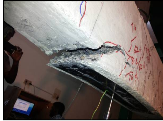
Fig. 10: Debonding of ASW-F specimen Fig. 11: Debonding of AFW-D specimen
