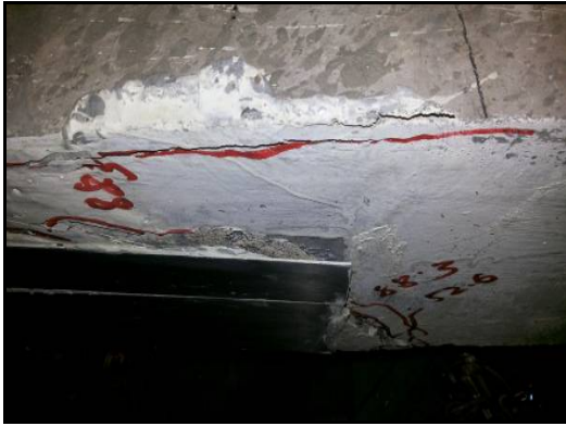
Fig. 10: Debonding of ASW-F specimen Fig. 11: Debonding of AFW-D specimen
