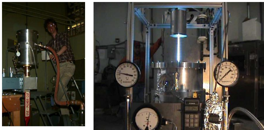
Figure 2 : The MET 75kW rocket engine operating with water propellant in air
