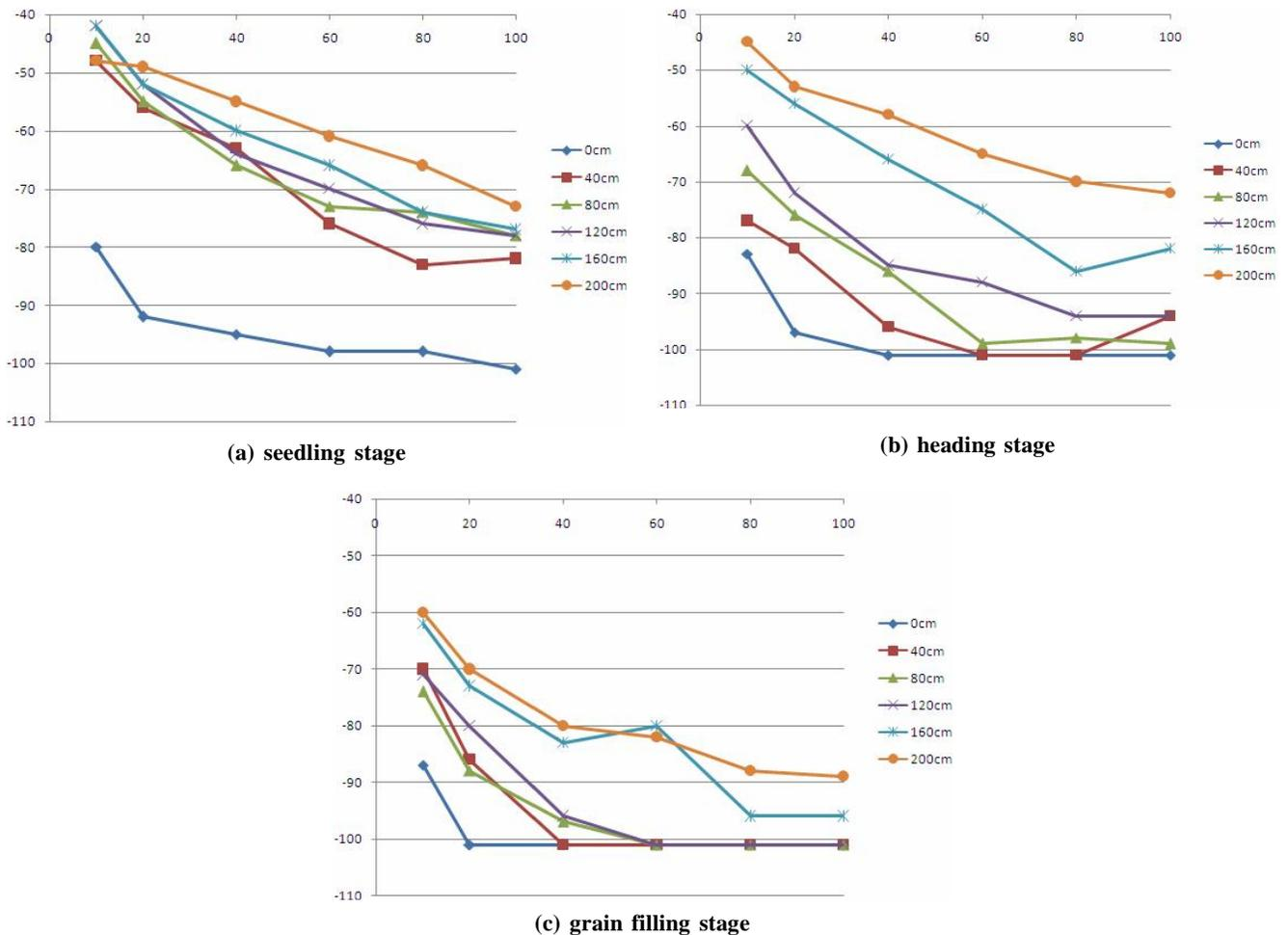
Figure 3 : The radio signal attenuation in different corn growth stage
