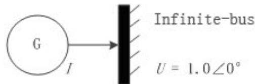
Figure 1 : Single machine infinite bus system
