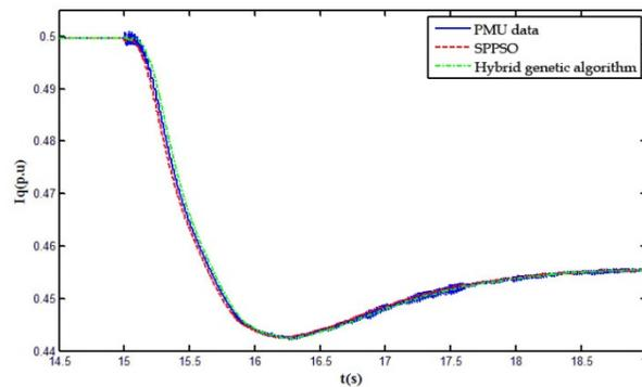
**Figure 4 : Comparison result of simulation data and PUM data of q axis**
