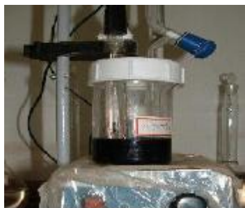
Figure 4: An electrochemical set up for Winkler’s iodometric titration in the same cell set up
