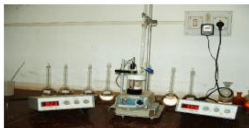
Figure 1: An electrochemical cell for DO measurement in water bodies
