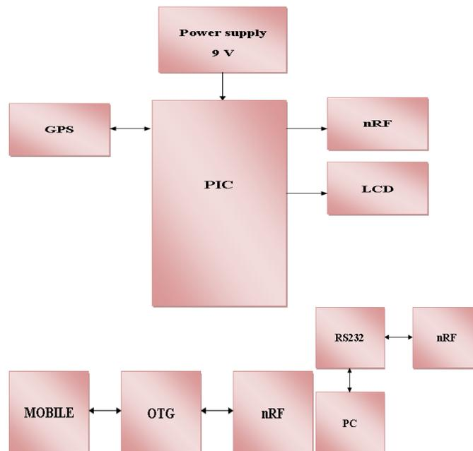
**Fig. 1: Block diagram of proposed system (patient, guardian and server section)**
