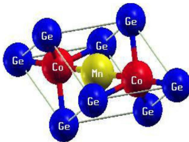
Figure 1 : Unit cell structure of  $\text{Co}_2\text{MnGe}$  Heusler alloy
