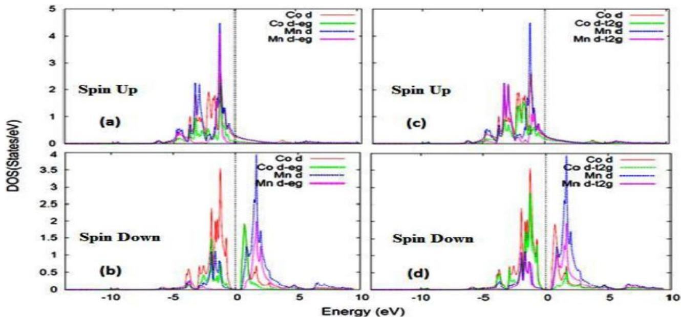
Figure 4 : DOS plots of  $\text{Co}_2\text{MnGe}$ , (a) Co (d, deg) and Mn (d, deg) states in spin-up; (b) Co (d, deg) and Mn (d, deg) states in spin-down; (c) Co (d, dt2g) and Mn (d, dt2g) states in spin-up; (d) Co (d, dt2g) and Mn (d, dt2g) states in spin-down
