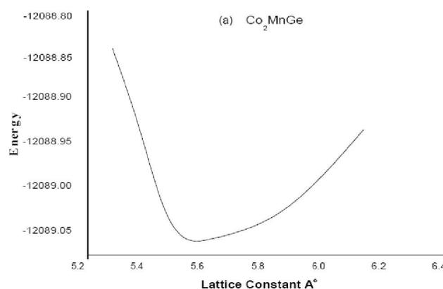
Figure 2 : Plot of energy versus lattice constant:  $\text{Co}_2\text{MnGe}$
