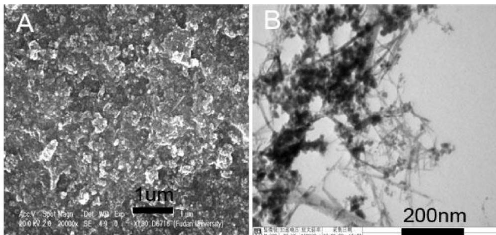
**Figure 2 :** The SEM image (A) and TEM image (B) of the typical  $\text{Fe}_3\text{O}_4$  @ PFR sample.
