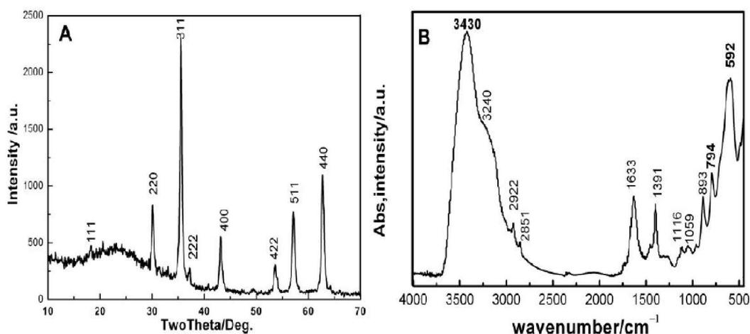
**Figure 1 :** The typical XRD Pattern (A) and FTIR curve (B) of the as-obtained  $\text{Fe}_3\text{O}_4$  coated by water-soluble PFR nanoparticles.
