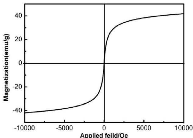
**Figure 3 :** Room-temperature VSM curves of the typical  $\text{Fe}_3\text{O}_4$  @ PFR samples.
