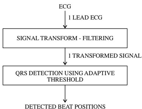
**Fig. 2: Pan-Tompkins beat detection algorithm work flow**
