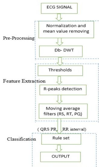
**Fig. 1: Block diagram of algorithm**
