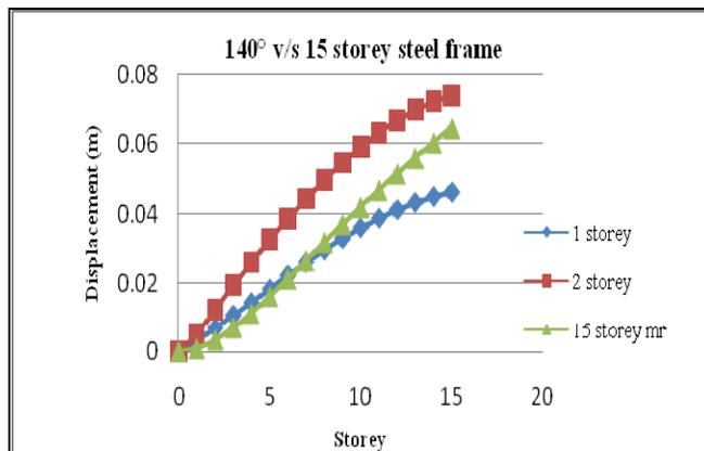
**Fig. 7: Displacement profile of 140°**
