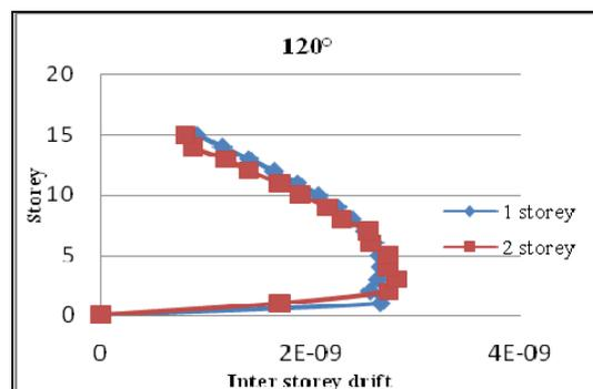
**Fig. 10: Interstorey drift profile of  $120^\circ$**
