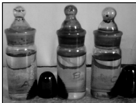
Fig. 1: Synthesized IONPs (A) Uncoated (B) Olive oil stabilized and (C) Linseed oil stabilized
