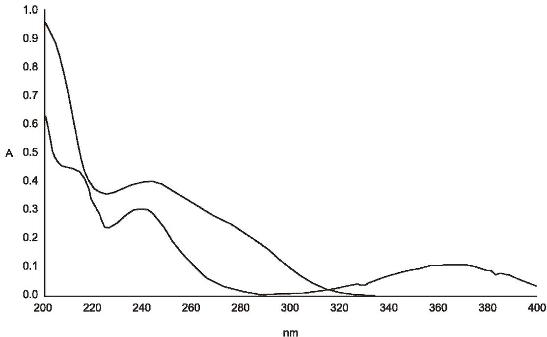
**Fig. 1: UV Spectra of 10 µg/mL of amlodipine and 10 µg/mL atorvastatin in methanol**
