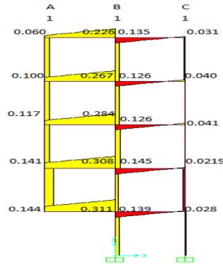
Fig. 5(i): Demand capacity ratio shear force (DCR) for longitudinal side of five-story bare frame building (Corner column removal scenario)
