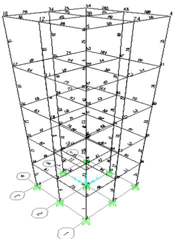
**Fig. 4: Nodes and beams nos of the building**
