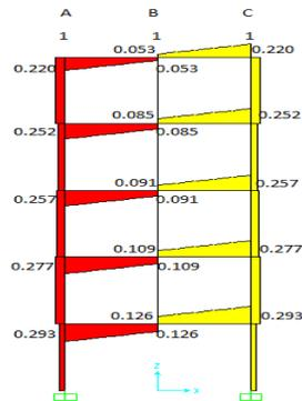
Fig. 5 (k): Demand capacity ratio shear force (DCR) for longitudinal side of five-story bare frame building (middle column removal scenario)
