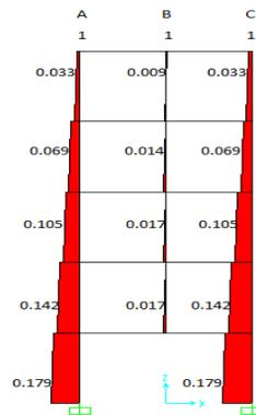
**Fig. 5(c): Demand capacity ratio axial (DCR) for longitudinal side of five-story bare frame building (middle column removal scenario)**
