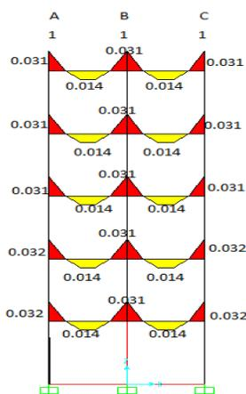
**Fig. 5(h): Demand capacity ratio bending moment (DCR) for longitudinal side of five-story with infill frame building (middle column removal scenario)**
