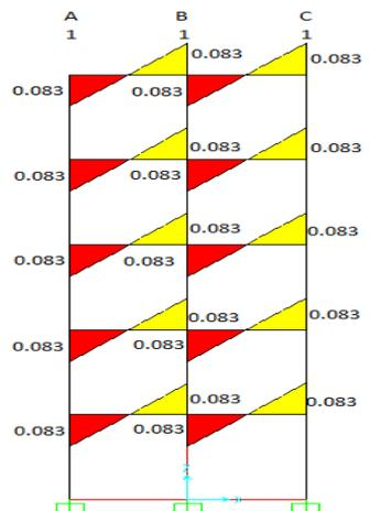
**Fig. 5(i): Demand capacity ratio shear force (DCR) for longitudinal side of five-story with infill frame building (middle column removal scenario)**
