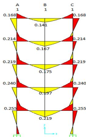
**Fig. 5(g): Demand capacity ratio bending moment (DCR) for longitudinal side of five-story bare frame building (middle column removal scenario)**
