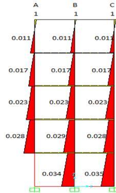
**Fig. 5(b): Demand capacity ratio axial (DCR) for longitudinal side of five-story with infill frame building (Corner column removal scenario)**
