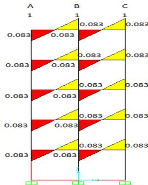
Fig. 5(j): Demand capacity ratio shear force (DCR) for longitudinal side of five-story with infill frame building (Corner column removal scenario)
