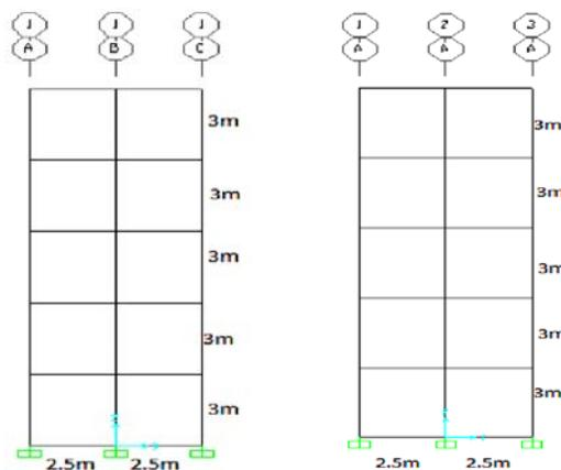
**Fig. 2: Front and side elevation of the building**
