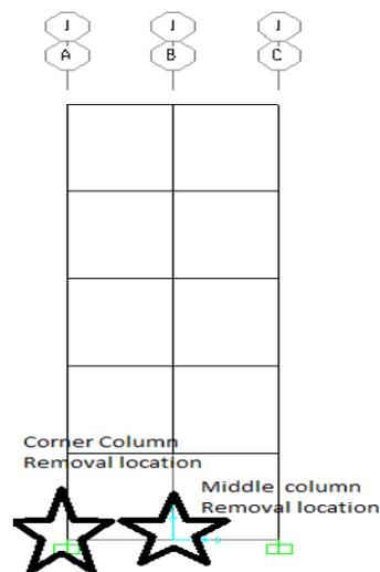
**Fig. 3: Diferent column removal location**
