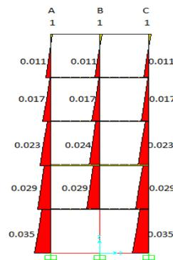
**Fig. 5(d): Demand capacity ratio axial (DCR) for longitudinal side of five-story with infill frame building (middle column removal scenario)**
