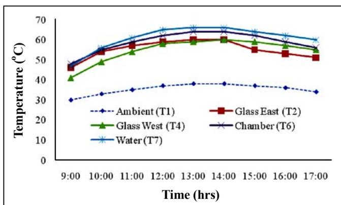
Fig. 3: Variation of temperature for 20 mm depth of water without PCM
