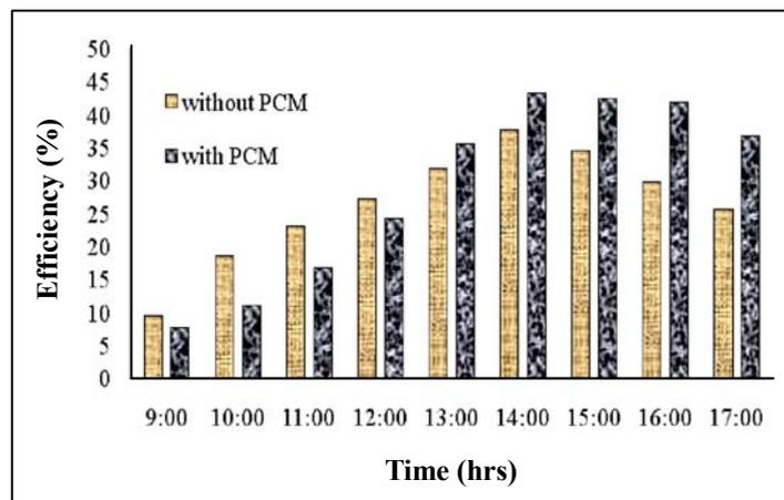
**Fig. 8: Variation of instantaneous thermal efficiency with time**
