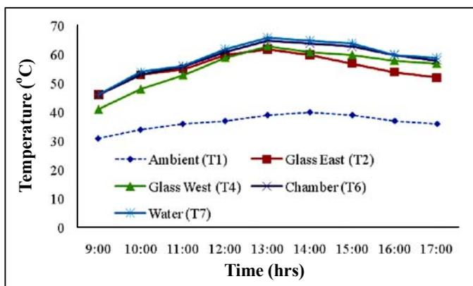
Fig. 4: Variation of temperature for 30 mm depth of water without PCM
