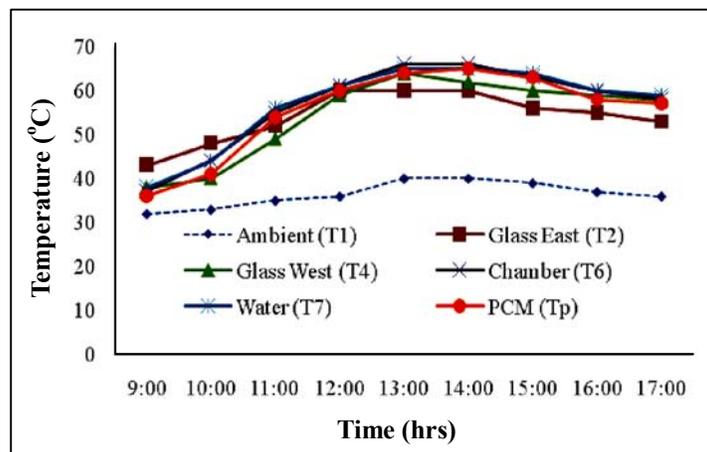
**Fig. 7: Variation of temperature for 30 mm depth of water with PCM**
