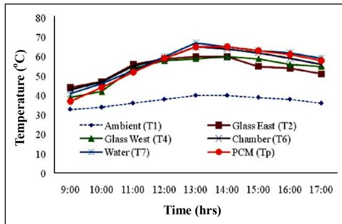
**Fig. 6: Variation of temperature for 20 mm depth of water with PCM**
