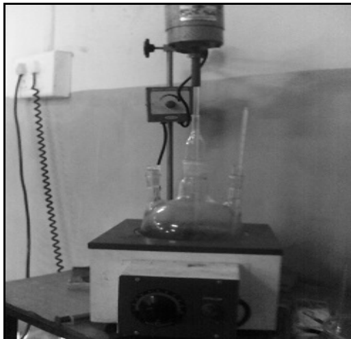
Fig. 1: Experimental set-up for bio-diesel production
