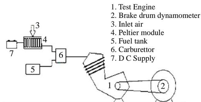
**Fig. 1: Schematic diagram of the experimental set up**
