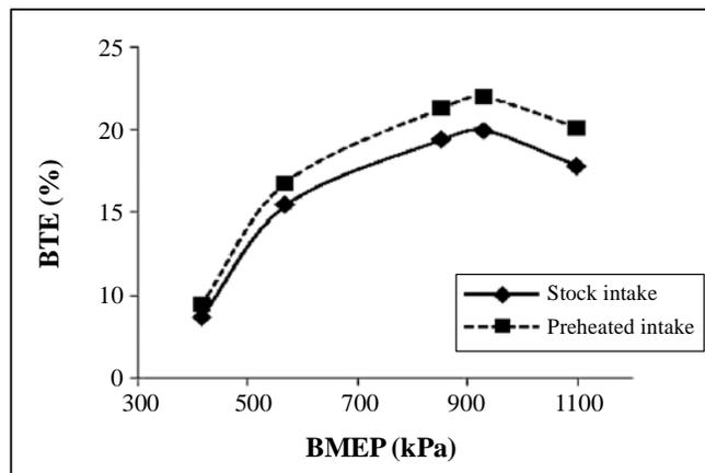
**Fig. 6: Variation of BTE with respect to BMEP**
