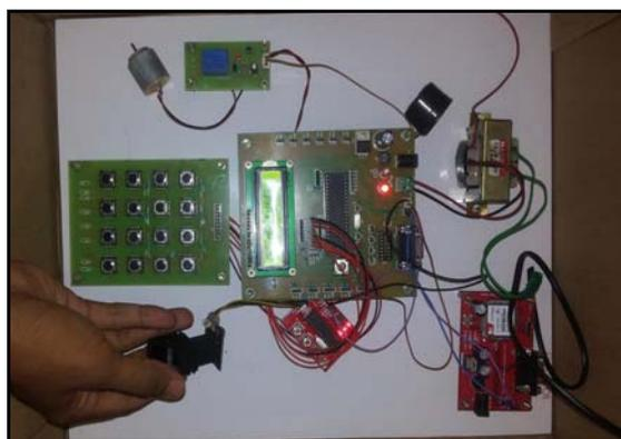
**Fig. 2: The hardware of fingerprint based ATM**
