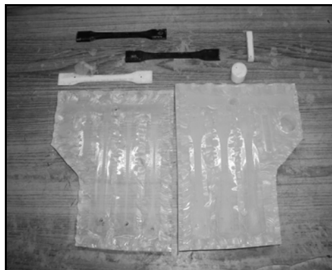
Fig. 4: Mold pattern with masters
