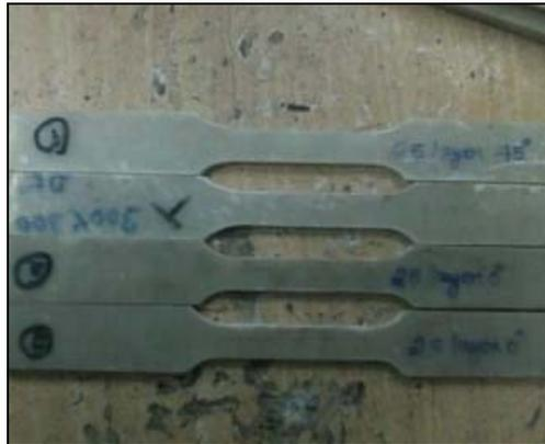
**Fig. 3.1: Tensile test specimen**
