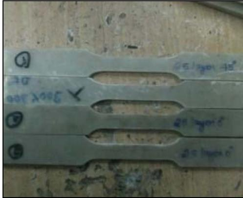
**Fig. 3.1: Tensile test specimen**
