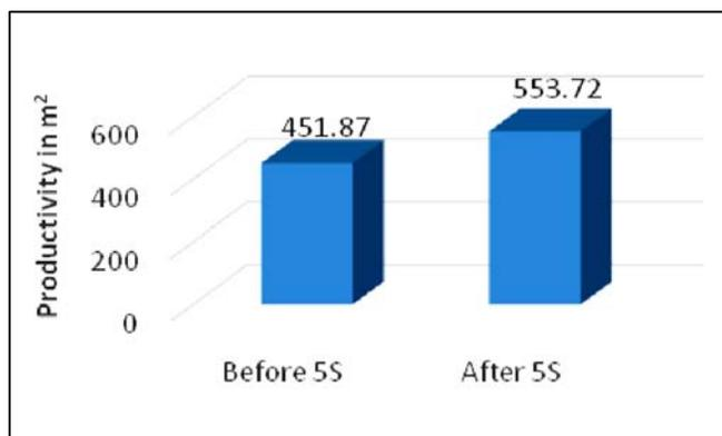
**Fig. 2: Productivity difference in external plastering for 58 masons before and after implementing 5S**
