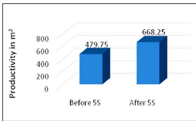
**Fig. 1: Productivity difference in internal plastering for 65 masons before and after implementing 5S**
