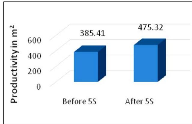
**Fig. 3: Productivity difference in ceiling plastering for 46 masons before and after implementing 5S**
