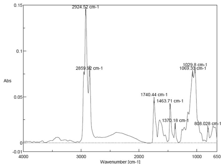
**Fig. 1: Fourier-transform infrared (FT-IR) spectra of pure mcl-PHA extracted from *P. putida***
