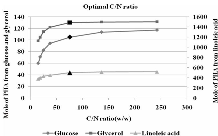
**Fig. 2: Simulation of various C/N ratio for higher yield of PHA using metabolic flux model**
