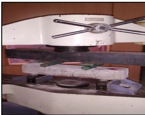
**Fig. 4: Flexural strength testing set up**
