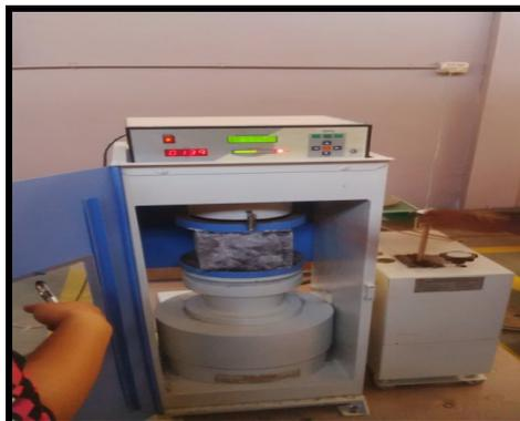
**Fig. 1: Compressive strength testing set up**
