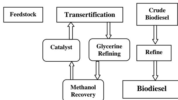
**Fig. 1: Conversion process of biodiesel production.**
