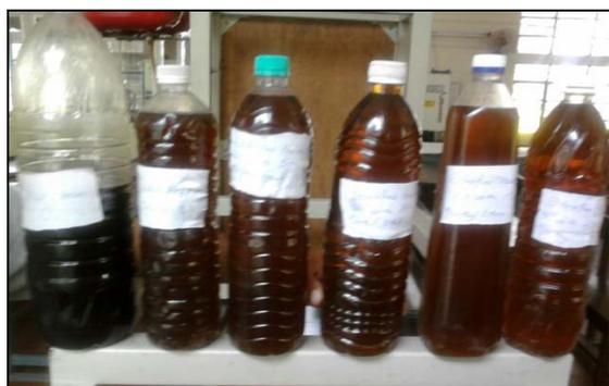
**Fig. 2: Blends of neem oil methyl ester with  $Al_2O_3$  nano**
