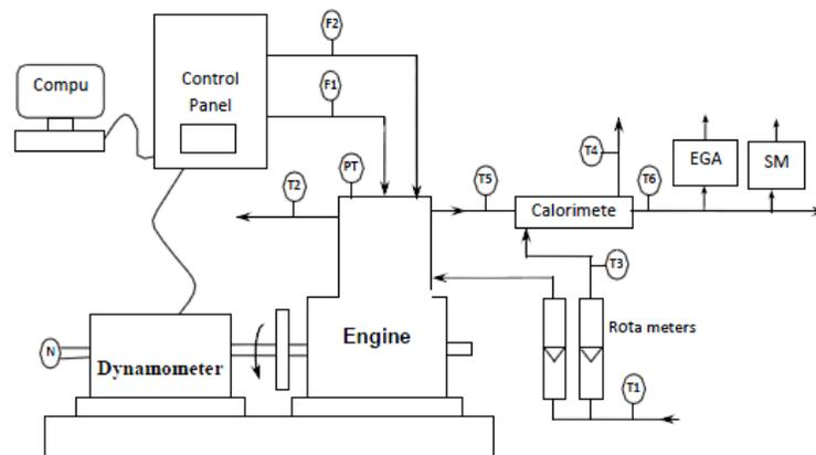
**Fig. 3: Experimental setup**
