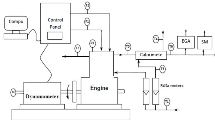
**Fig. 3: Experimental setup**
