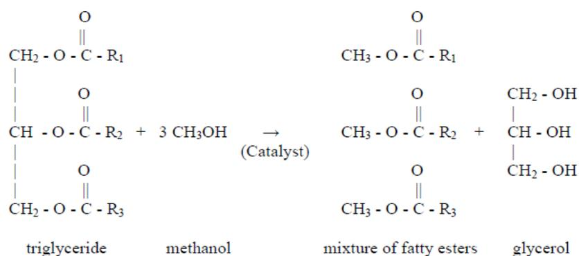
**Fig. 1: Transesterification chemical reaction**
