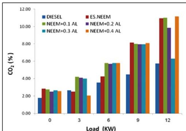
**Fig. 5: Variation of CO<sub>2</sub> on Load**
