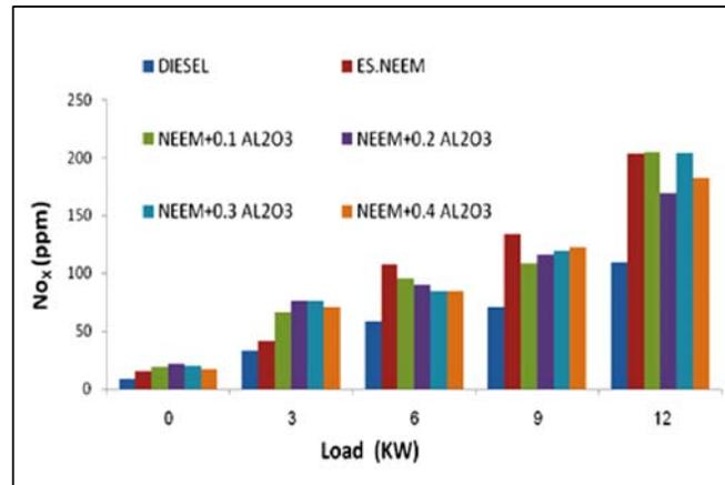
**Fig. 3: Variation of  $\text{NO}_x$  on Load**
