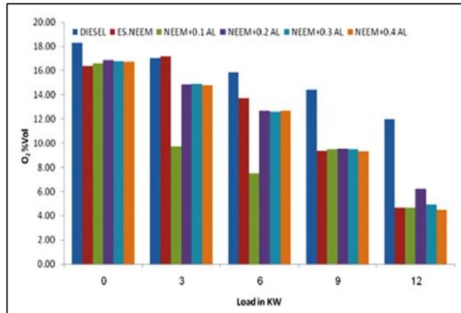
**Fig. 7: Variation of O<sub>2</sub> on load**
