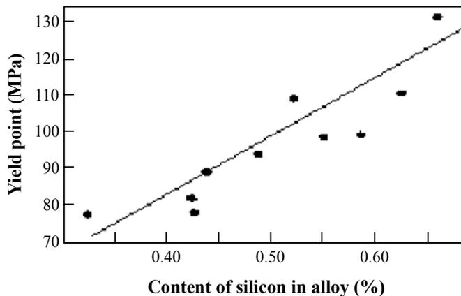
**Fig. 2: Dependence of the yield point strength of AD31 aluminum alloy on silicon content**
