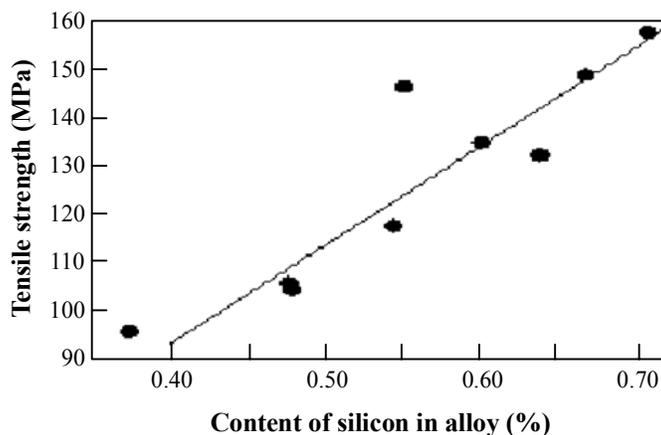
**Fig. 3: Dependence of tensile strength of AD31 aluminum alloy on silicon content**
