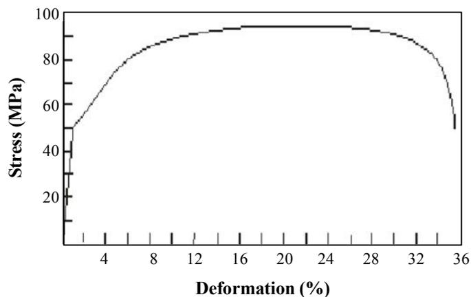
**Fig. 1: Aluminum sample tensile stress-strain diagram after annealing**
