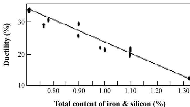
**Fig. 7: Dependence of ductility on the total content of iron and silicon in AD31 aluminum alloy**
