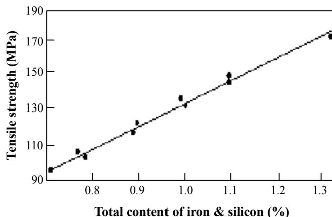
**Fig. 6: Dependence of tensile strength on the total content of iron and silicon in AD31 aluminum alloy**
