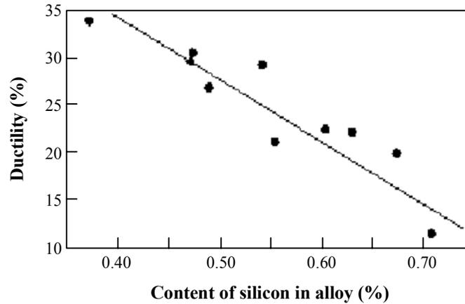
**Fig. 4: Dependence of ductility margin of AD31 aluminum alloy on silicon content**
