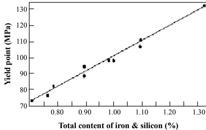
**Fig. 5: Dependence of the yield point on the total content of iron and silicon in AD31 aluminum alloy**
