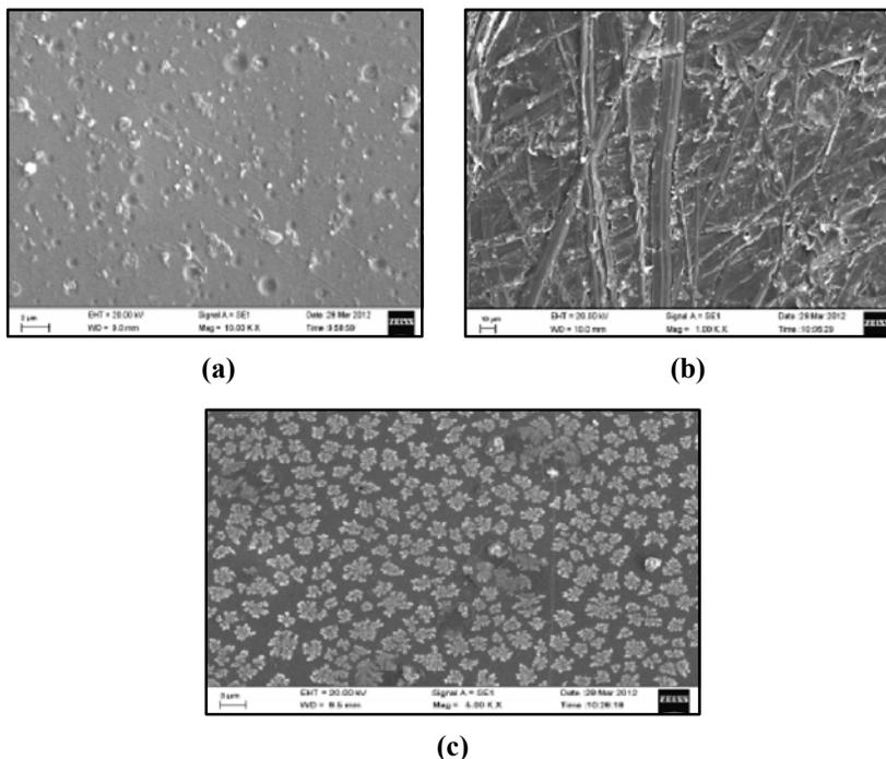
**Fig. 5: SEM images for (a) PS, (b) 0.01 MWNT/PS and (c) 0.05 MWNT/PS nanocomposites**
