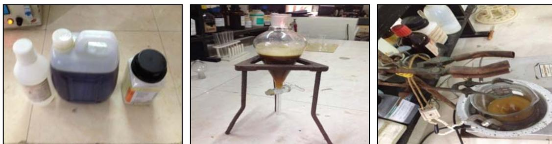
**Fig. 1: Raw jatropha oil, methanol & catalyst, separating funnel, flask cum stirrer & external heater**
