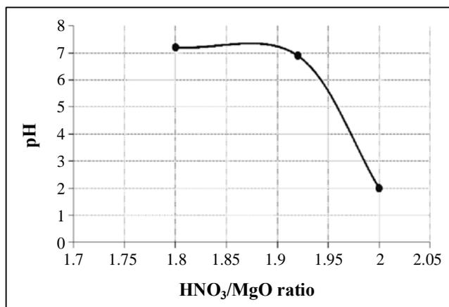
**Fig. 2: Final product pH as a function of the ratio  $\text{HNO}_3/\text{MgO}$**
