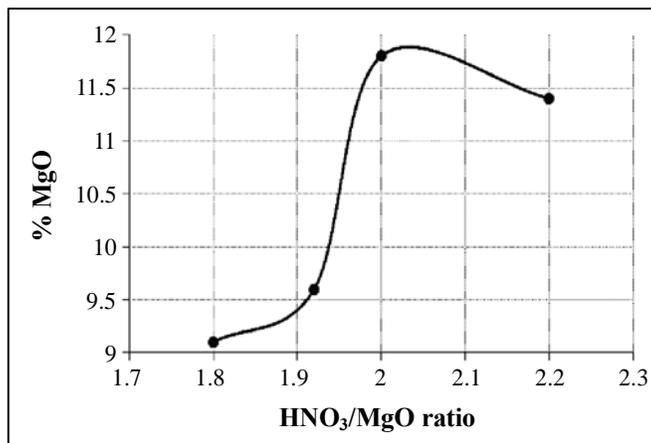
**Fig. 3: Final product MgO percentages as a function of the ratio HNO<sub>3</sub>/MgO**
