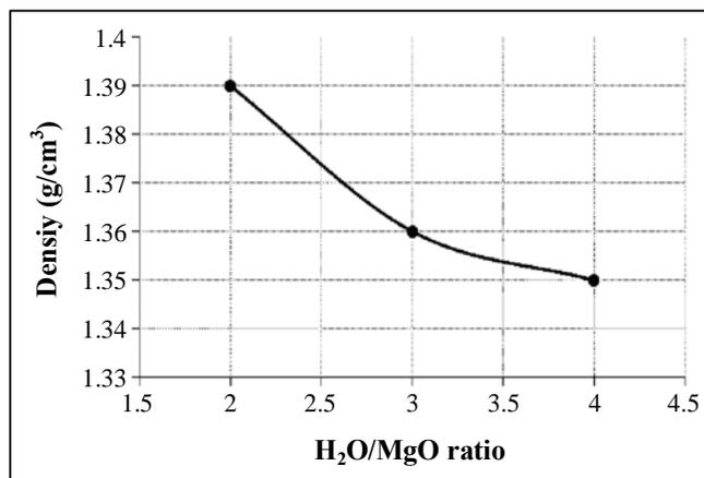
**Fig. 1: Final product density as a function of the ratio  $\text{H}_2\text{O}/\text{MgO}$**
